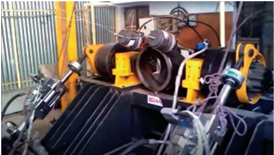
Figure 25 Testing truck braking system
