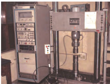
Figure 2 IMTC controller on an MTS test system at IISc (c. 1986).
