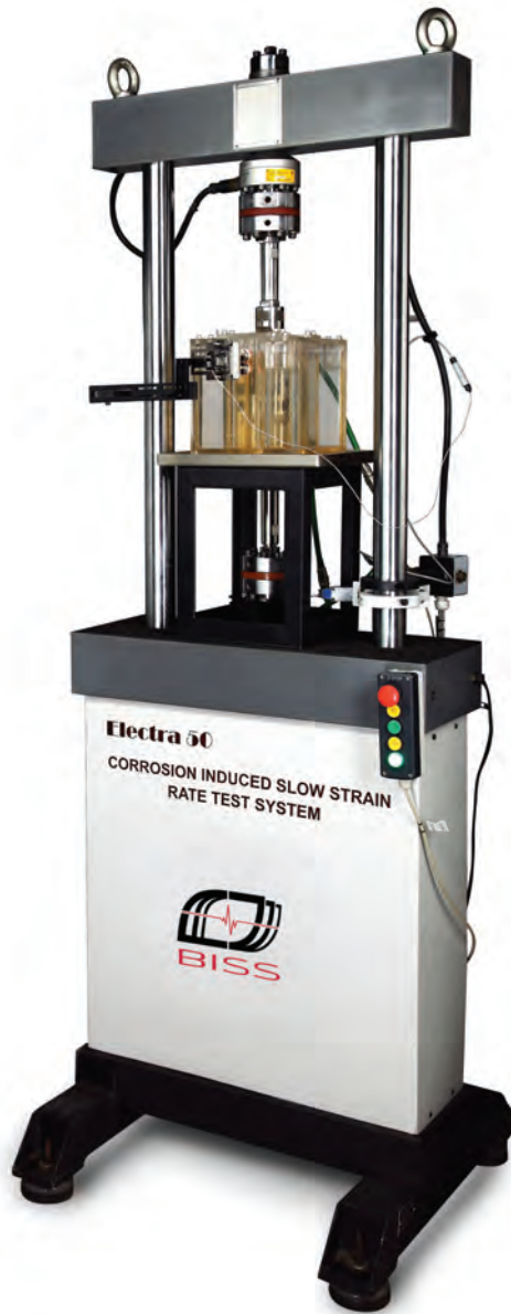
Figure 41 Corrosion induced LCF test system
