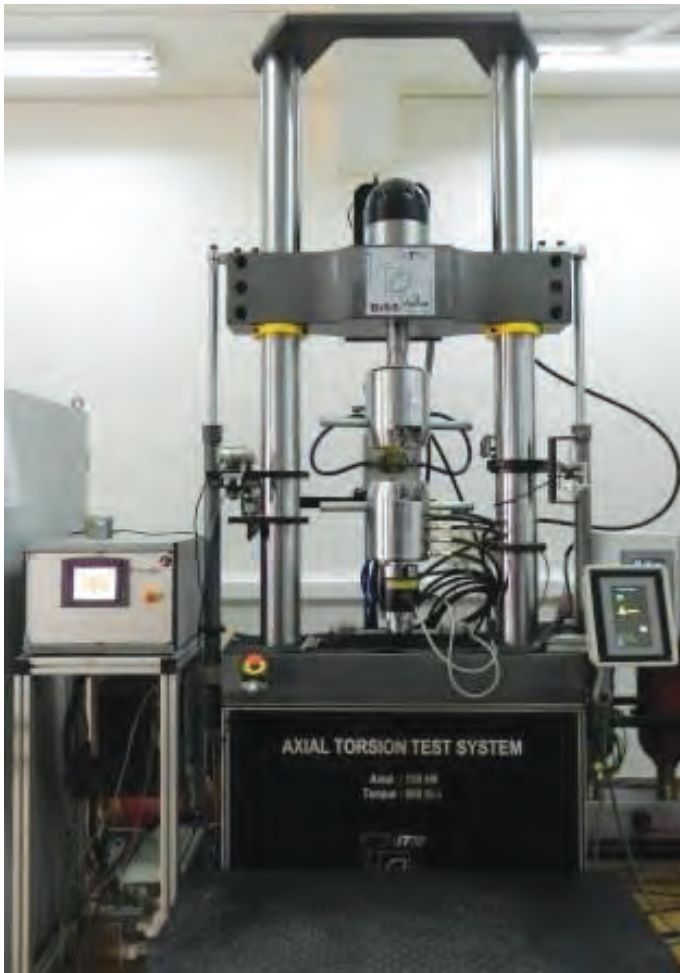
Figure 59 Figure 1 High Strain Rate ATTS system at IGCAR
