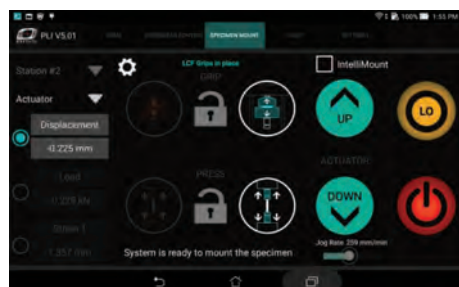
Figure 10 PLI App panel for adjusting actuator position for ease of specimen mounting.
