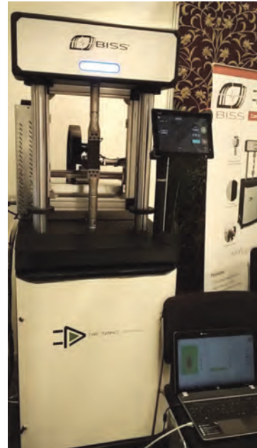
Figure 53 25 Nano static and fatigue test system with 3D online scanner for CFRP specimen.
