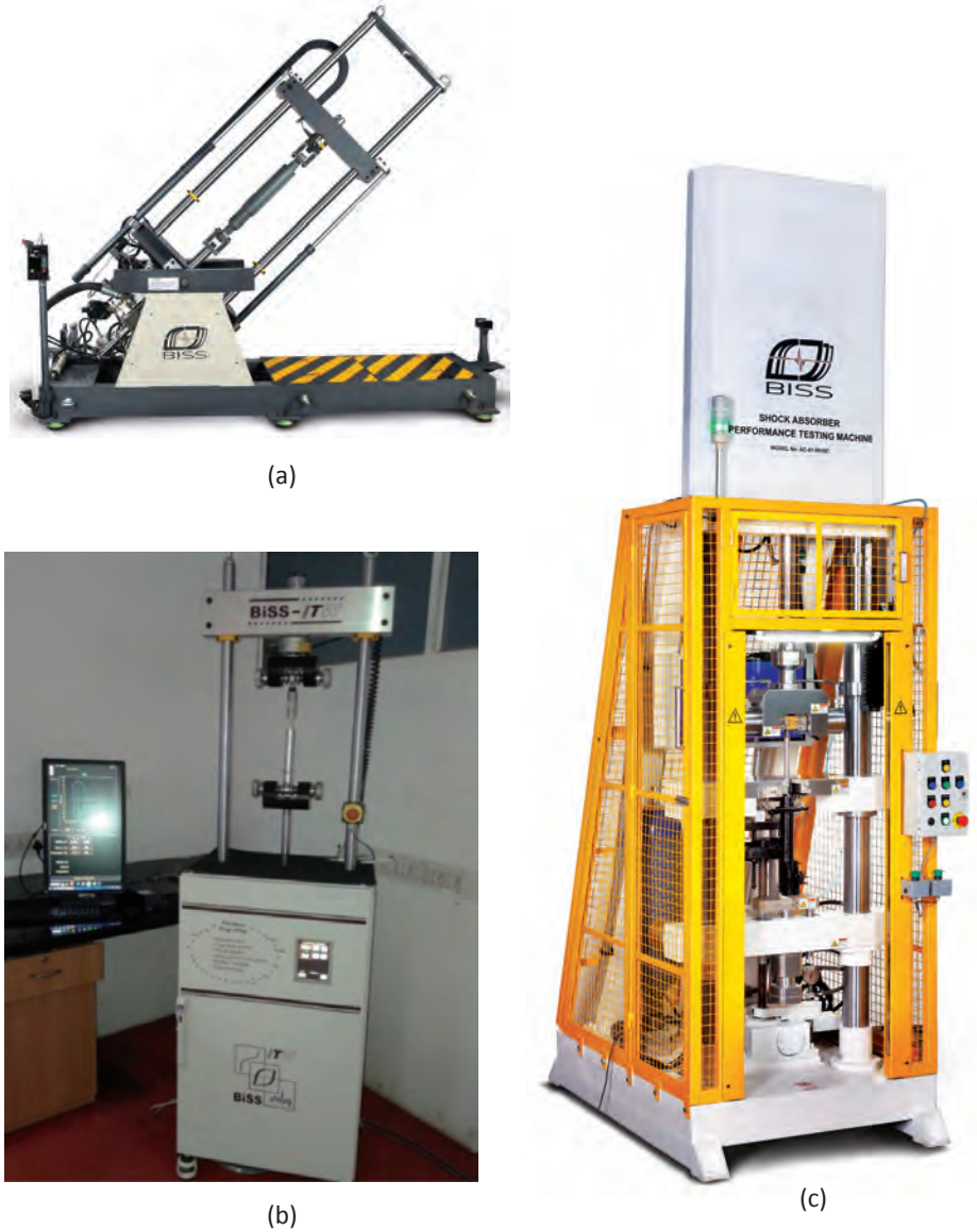
Figure 87 Various versions of shock absorber test systems; (a) System for testing at tilted position; (b) portable single station damper test system; (c) High speed damper test system.
