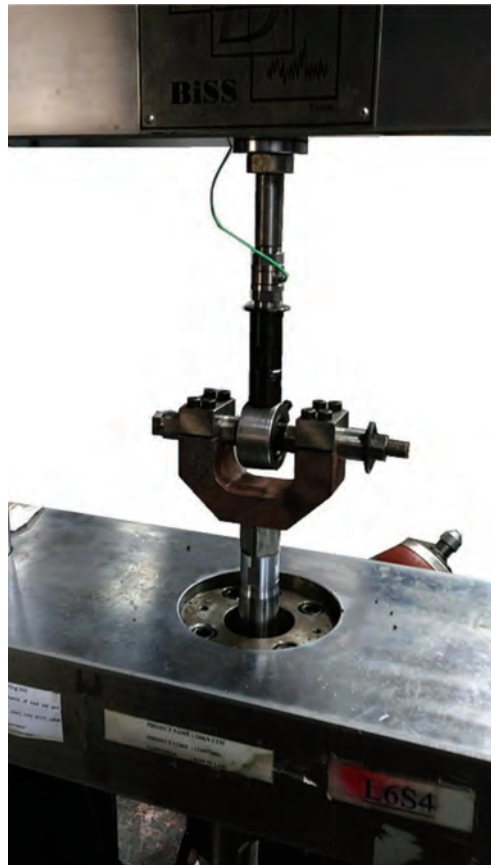
Figure 61 Elastomer test setup with piezoelectric loadcell.
