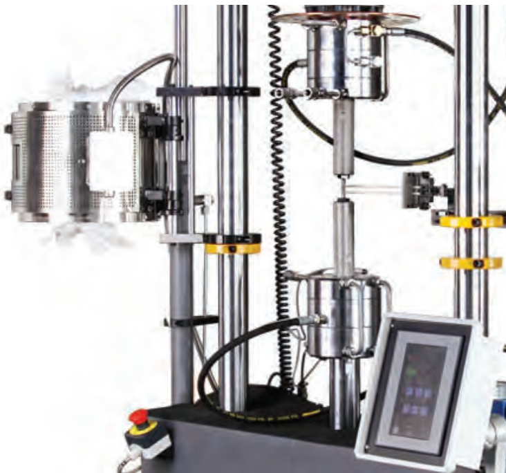
Figure 34 LCF test facility with high temperature furnace, grips and extensometer.
