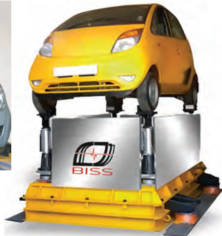
Figure 19 Four-poster test rig for dynamic testing of vehicle structure for road loads.
