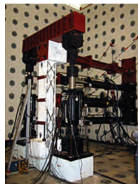
Figure 6 High performance actuators (2000kN), at NTU Singapore, retrofitted with BISS 2370 controller
