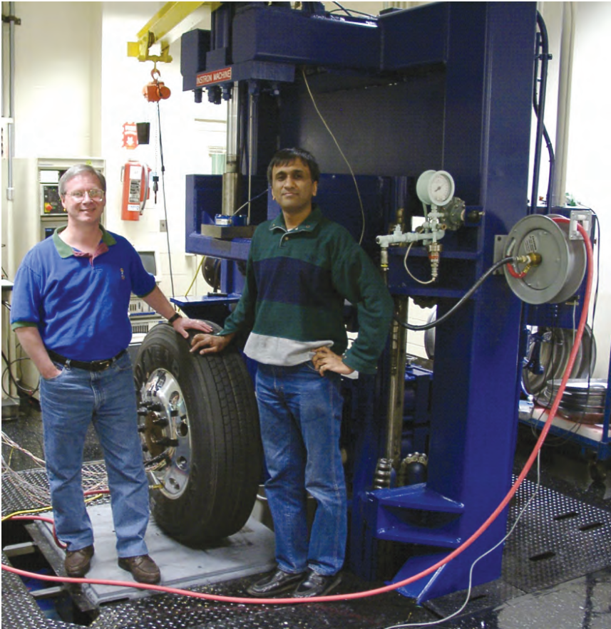
Figure 26 Triaxial wheel tester at Accuride Inc. USA.
