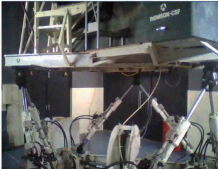
Figure 27 6-actuator flight simulator with Indian Air Force.
