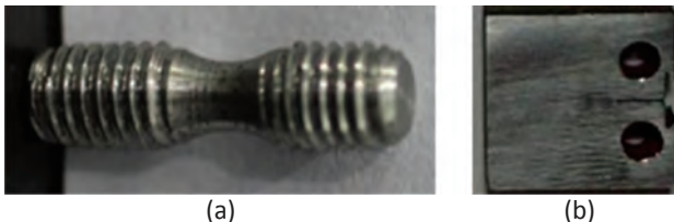
Figure 68 Miniature specimens tested on BISS low force test systems: (a) tensile / LCF specimen (M5 mm, GL 3mm); and (b) Fracture toughness / Fatigue crack growth (W12 mm, T5 mm).
