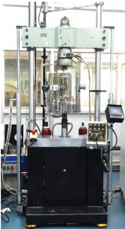
Figure 56 100kN High Strain Rate test system at IGCAR.
