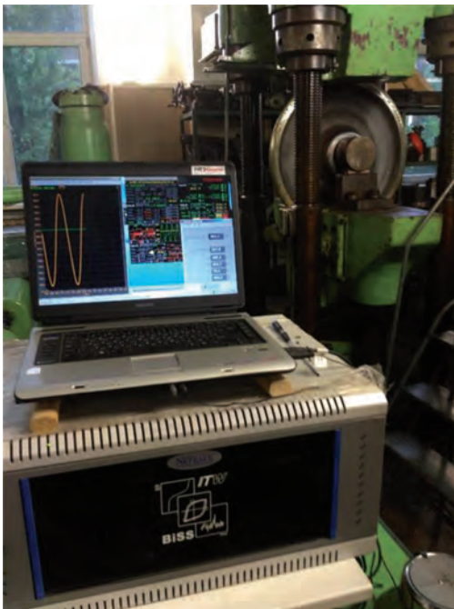
Figure 28 300-ton wheel test system with pulsator at the Federal Research Institute of the Russian Railways.
